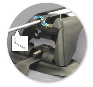
Tighten adjusting screw to 5 Nm (3.7 ft lb) hand tight.
